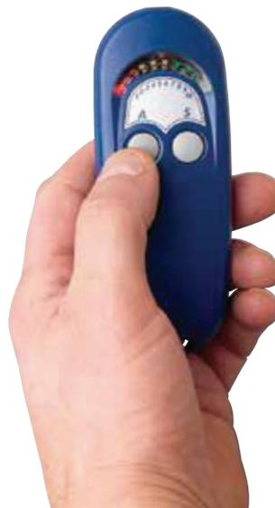
A UVA Meter can quickly and clearly show the condition and quality of the UV output of existing tubes in a fly trap, showing whether they are working at peak performance, in need of replacement or beyond useful life.
