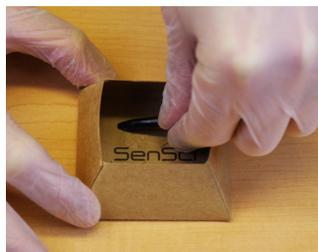
Place Activ<sup>CR</sup>™ vial on the inner capture surface and press vial to the glue to secure the vial.
